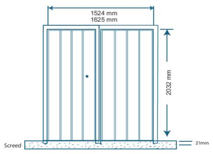
Widths are into rebate of frames. Heights are from finished floor to head rebate.
